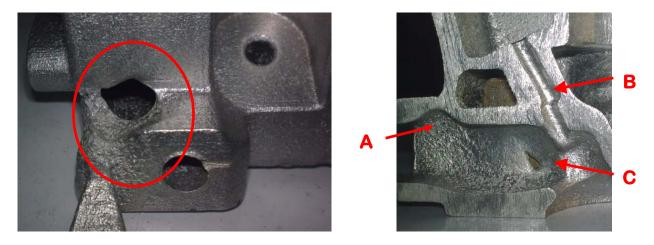
Figure 14. Shrinkage defects surrounding massive regions of the part
