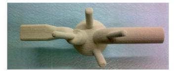
Figure 10. Combustion chamber, inlet and exhaust passages inner core (note the swirl geometry)
