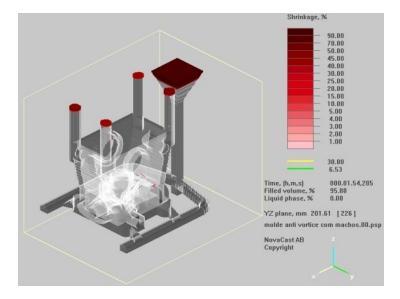
Figure 13. NovaCast® shrinkage prediction
