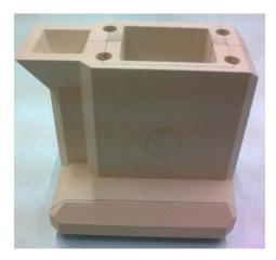
Figure 12. Fully assembled mould ready for metal pouring
