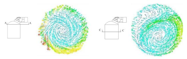
Figure 6. Final geometry with FLUENT (swirl) results at two locations of the cylinder
