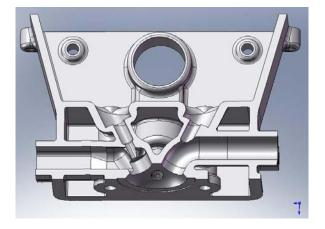
Figure 15. Design #3 – Bottom isometric view (left) and half cut showing the new coolant chamber (right)
