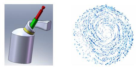
Figure 3. Initial inlet passage design and produced swirl inside the cylinder
