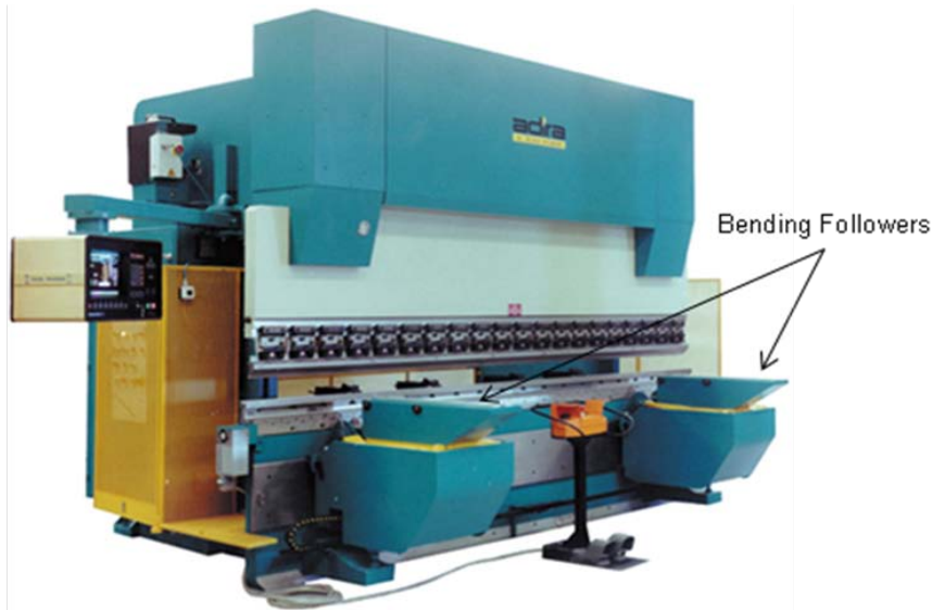
Figure 2.1: Press brake ADIRA - QIHD with bending followers.
