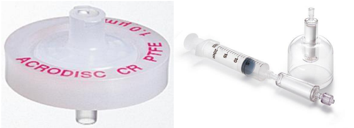
Figure 4 – Enclosed filter examples
