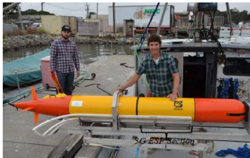
Figure 9 – 3G-ESP mounted in an AUV
