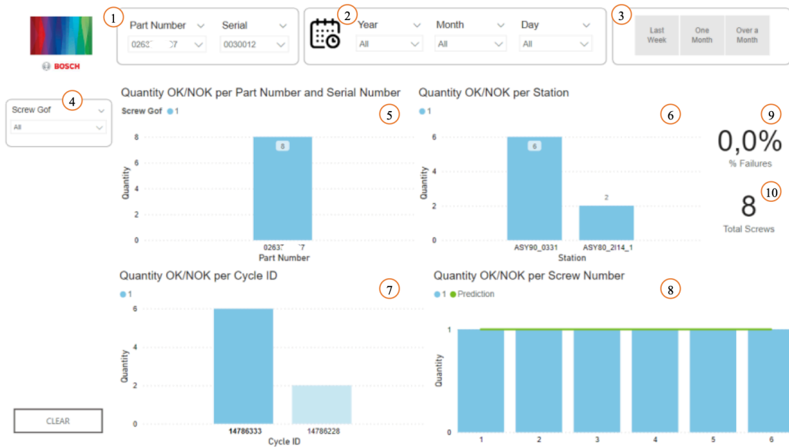
Figure 24: Detailed Screw Tightening dashboard with GoF 0, from Galvão et al. (2022).
