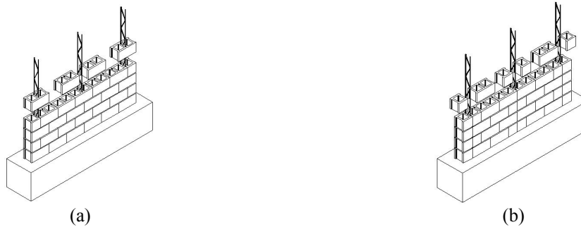
Figure 4: Masonry bonds: (a) running masonry bond, B1 (b) bond with continuous vertical joint, B2
