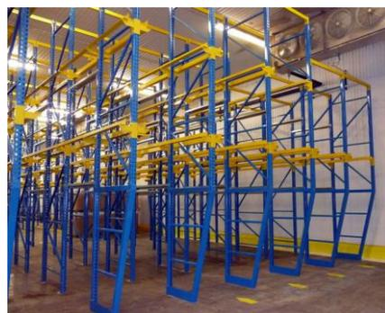
Figura 5 - Rack drive-through (REB Storage Systems International, 2023).
