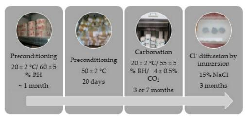
Figure 5. Scheme for combining tests to study the effect of carbonation on the penetration of chlorides.
