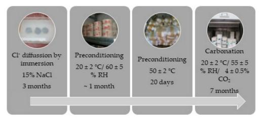
Figure 4. Scheme for combining tests to study the effect of the presence of chlorides on carbonation.
