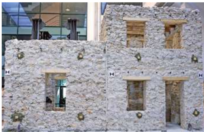
Fig. 2 – SERA AIMS specimen before plastering (Tomić et al. 2022a).
