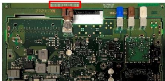
Figure 7: Example of a barcode in a PCB.
