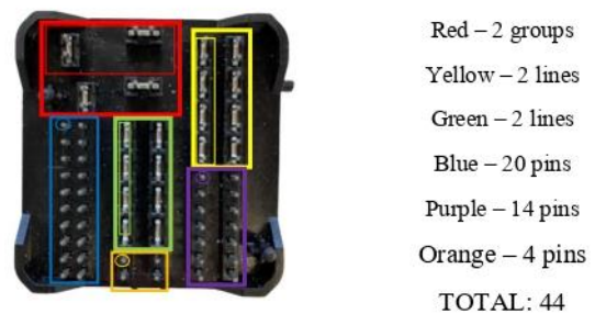
Figure 4 - Component divided into sections and number of pins of each section.
