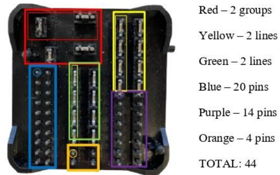
Figure 10: Component divided into sections and number of pins of each section.
