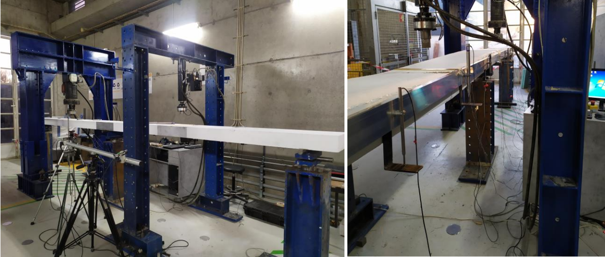
Figure 9 - Monitoring systems for measuring the deflection, reaction forces and average crack width in the sagging and hogging regions of the shallow beam: (a) Front view; (b) Rear view; and (c) Photo of the front and rear view of the prototype in the test setup (dimensions in mm).
