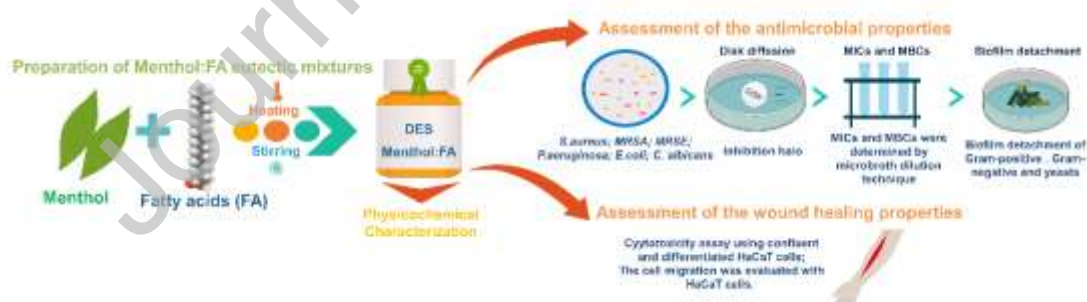
Figure 1. Schematic illustration of DES production steps, considering their physicochemical and bioactivity assessment.
