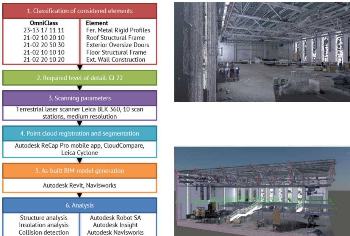
Figure 2 – Scheme of the proposed methodology, which is tuned for the case study for existing industrial sites and the as-Built model (Badenko et al., 2019)
