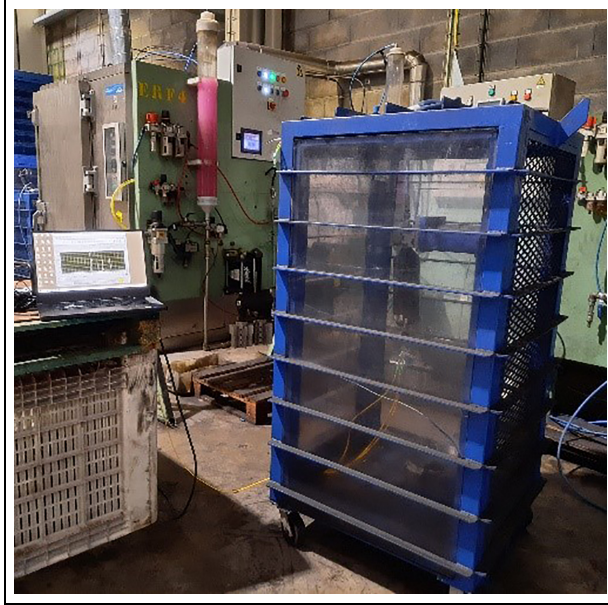
Figure 4. Cyclic pressure test and optical fibre monitoring setup at Amtrol-Alfa.
