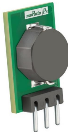
Figura 5.19 – Conversor OKI-78SR-3.3/1.5-W36-C da Murata Power Solutions .
