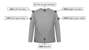
Fig. 1. IMUs position within the ergonomic vest.
