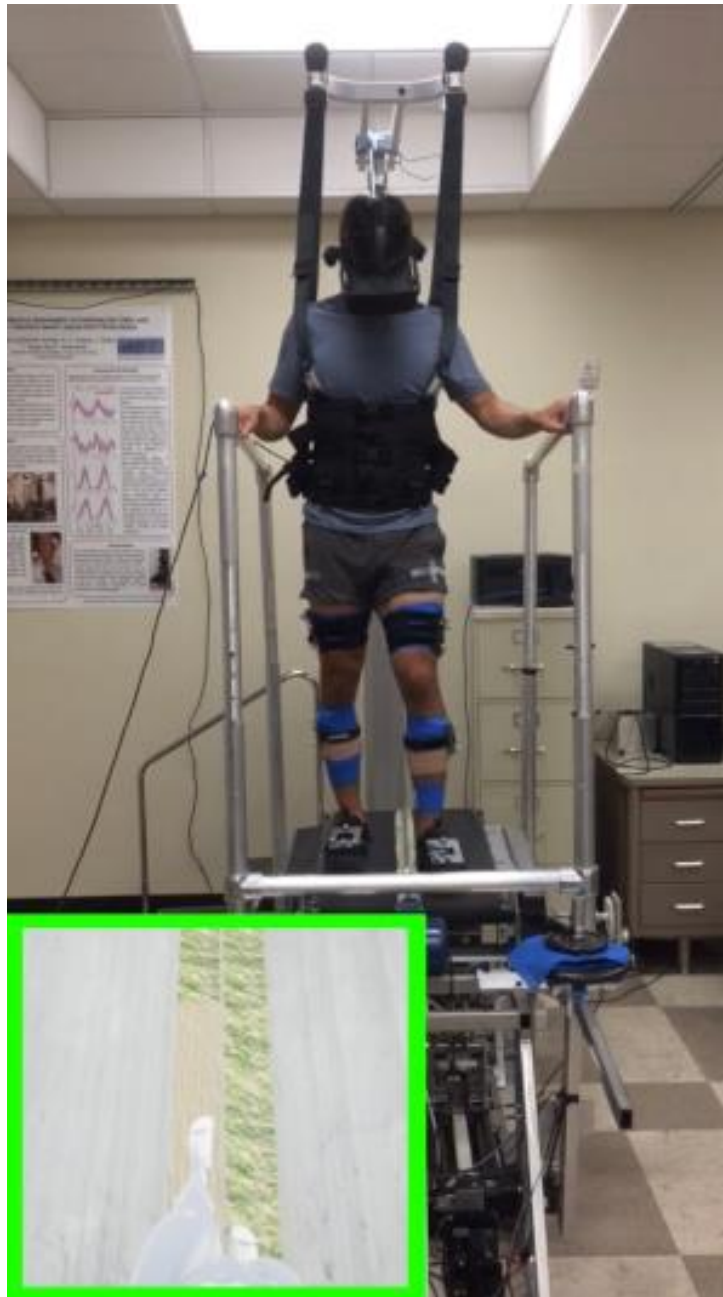
Figure 18: Figure from Drolet et al. [166] setup consisting of a treadmill of variable stiffness and virtual environment delivered by a HMD.
