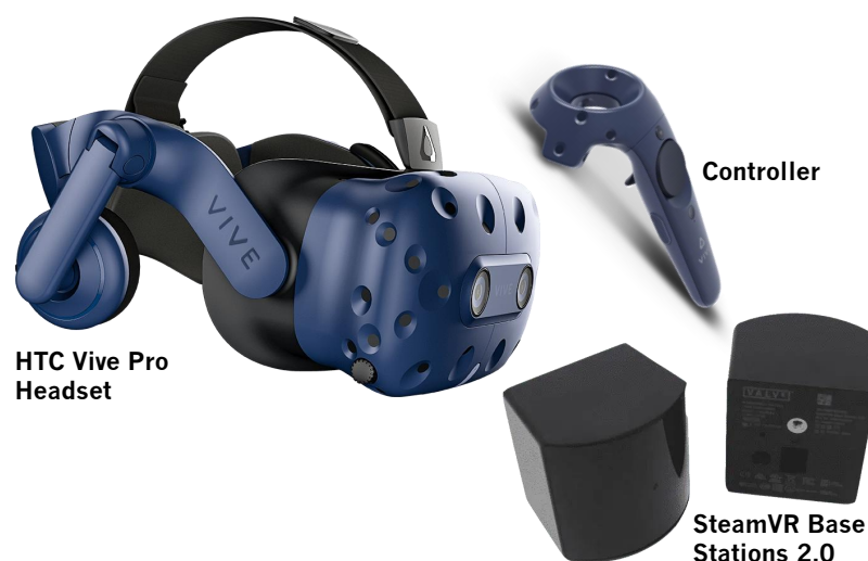
Figure 42: HTC VIVE Pro Full Kit. Images reproduced from [244]
