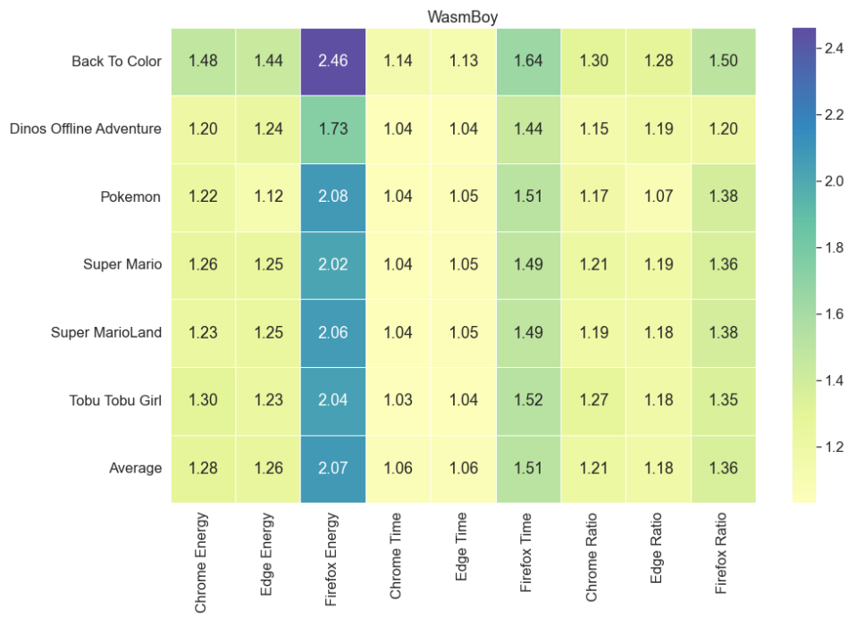
Figure A.7: WasmBoy: Heat map representing the proportion between WebAssembly and JavaScript results in the three browsers.
