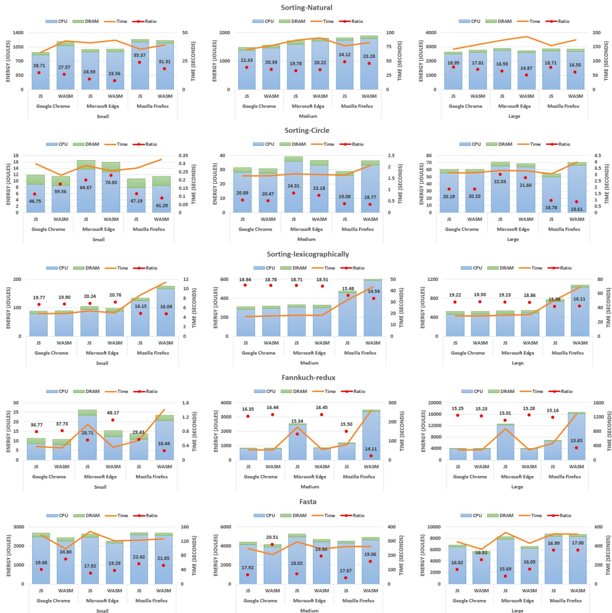
Figure 4.4: Energy consumed by each browser for each benchmark with the three input sizes and the respective execution times and ratio values.
