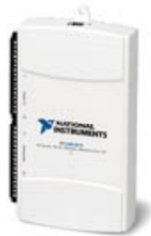
Figure 3.4 - NI USB-6210 DAQ board used in CaTraSys (National Instruments Corporation, 2009).
