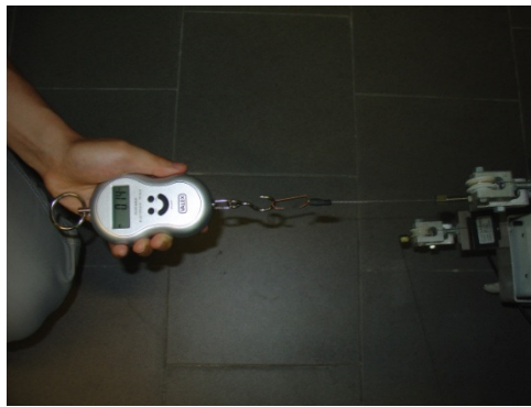
Figure 3.13 - Electronic scale device measuring the force exerted on the cable.
