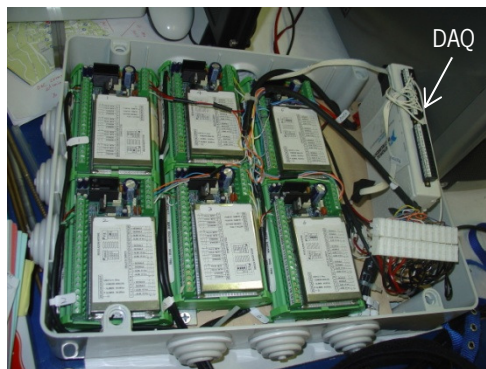
Figure 3.8 - The 6 amplifiers together with the DAQ board.
