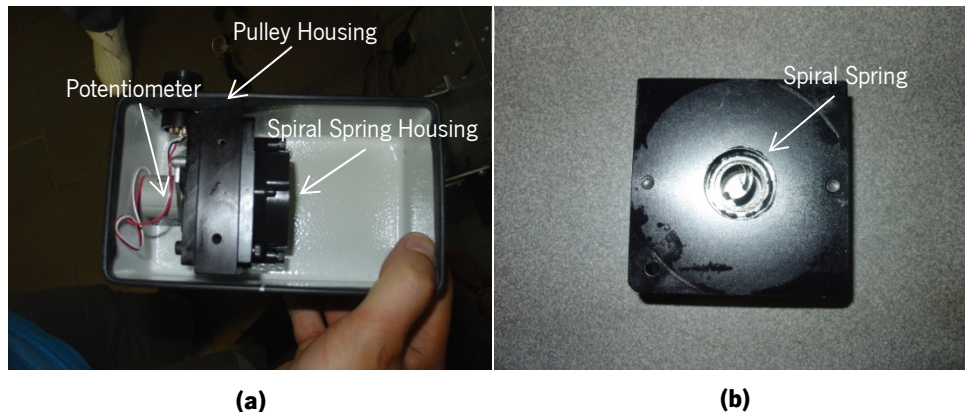
Figure 3.5 - Position transducer: (a) inside view of the plastic protective box; (b) spiral spring.
