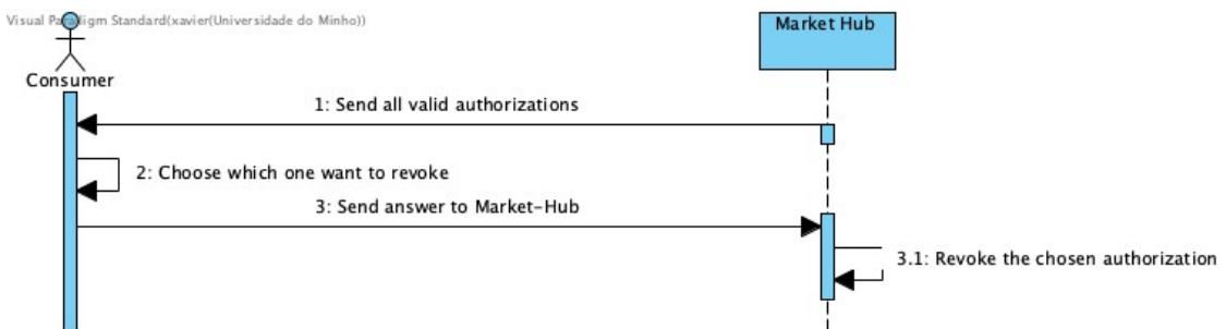
Figure 81: Revoke Authorization Subsystem Sequence Diagram
