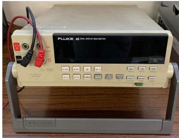
Figura 19. FLUKE 45 Dual Display Multimeter
