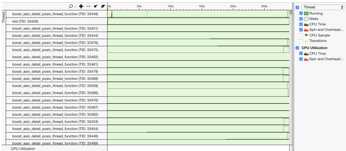
Figure 19: Thread state report from VTune
