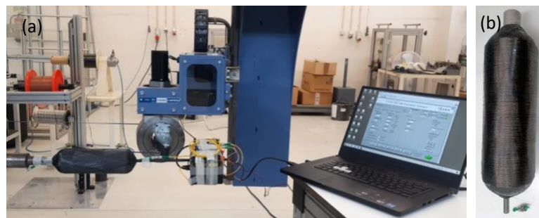
Figure 2: Production of the COPV by tape winding
