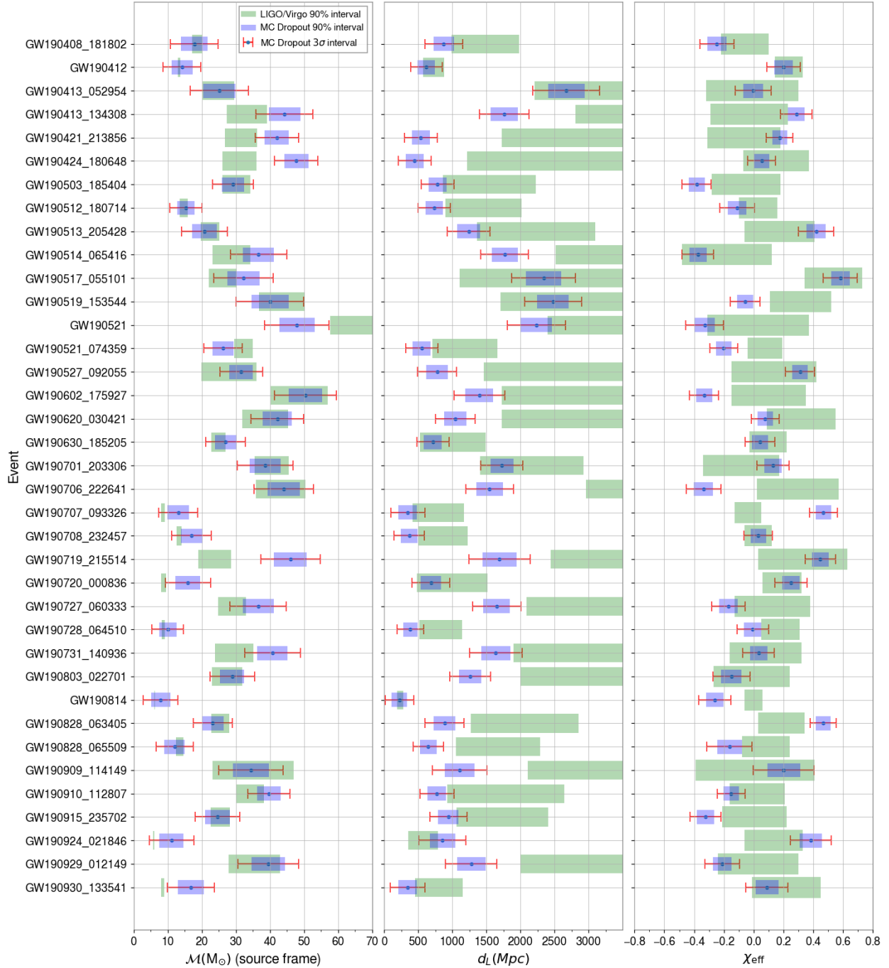
Figure 7.2: Best-performing DL network's prediction for the chirp mass (left), luminosity distance (middle) and effective inspiral spin (left) for the BBH events from GWTC-2.
