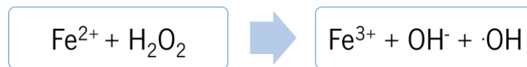
Figure 4. Fenton Reaction: hydrogen peroxide ( H_2O_2 ) oxidizes iron (II) ( Fe^{2+} ) into iron (III) ( Fe^{3+} ), hydroxyl radicals (OH) and hydroxide anions (OH).
