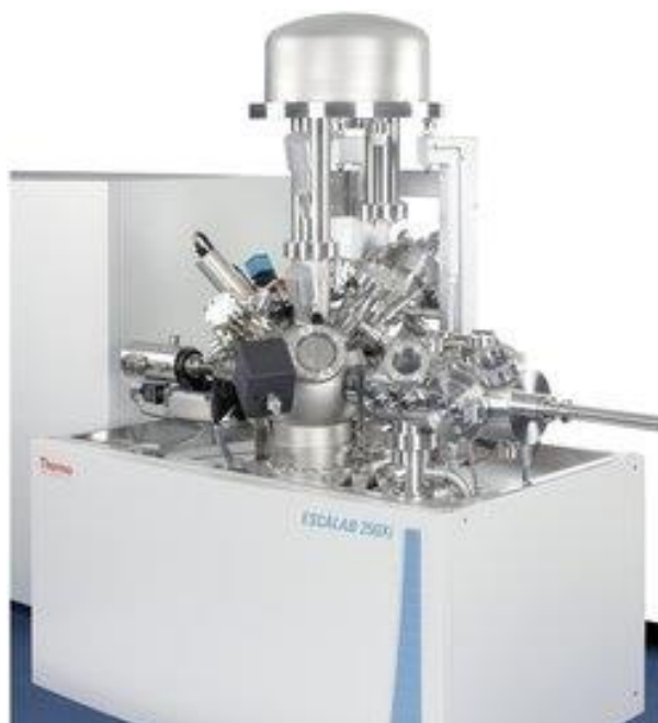
Figure 17. ESCALAB 250Xi X-ray photoelectron spectrometer (Thermo Scientific) used in this thesis work.
