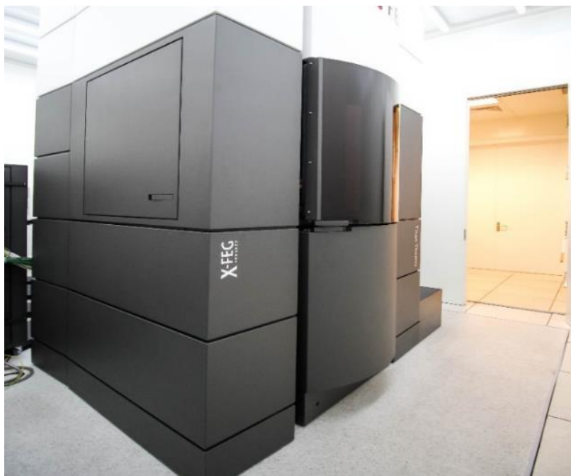
Figure 19. Double Corrected HRTEM - Titan Themis 60-300 kV used in this thesis work.
