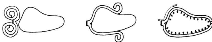
Figure 4 – Grasping phase of the soft gripper presented by Hirose, S. and Umetani, Y. [7]. The finger is initially at a resting position thanks to a releasing wire. Once the input torque is applied, the fingers envelop the object distributing the contact forces around the object.
