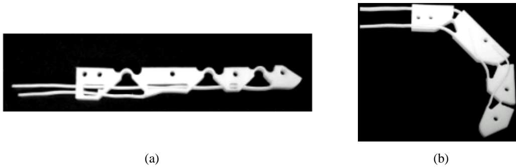
Figure 5 – Under-actuated finger composed by Teflon material [13]. The rigid joint coupling achieved by the one-piece structure allows reducing the cost of the manufacturing process – (a). The finger design determines the limit configuration angle for the bending motion of the three hinges – (b).
