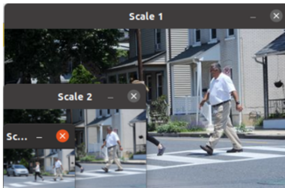
Figure 3.6: Image Pyramid algorithm for multiple scale detection.
