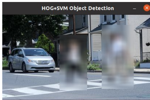
Figure 3.8: Blurring filter for anonymization of target object in Object Detection algorithms.
