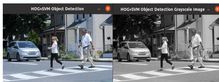
Figure 3.4: Grayscale transformation routine for Image Processing applications.
