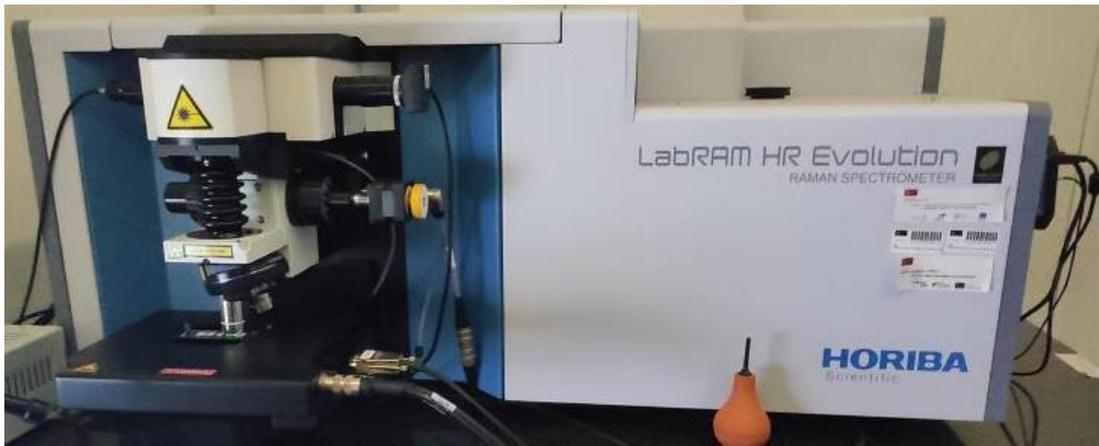
*Figura 18-Equipamento de Raman (LabRAM HR Evolution Raman Spectrometer).*
