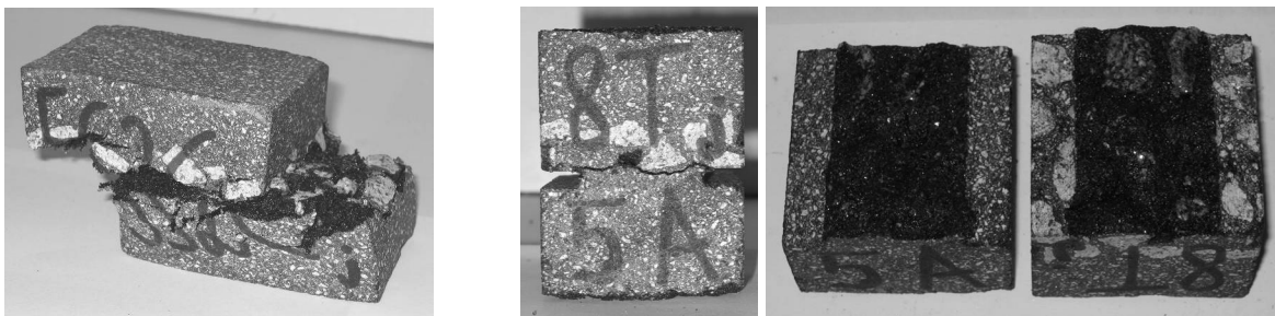
Figure 4. Rupture area observed in shear tests (left) and in tensile tests (right)
