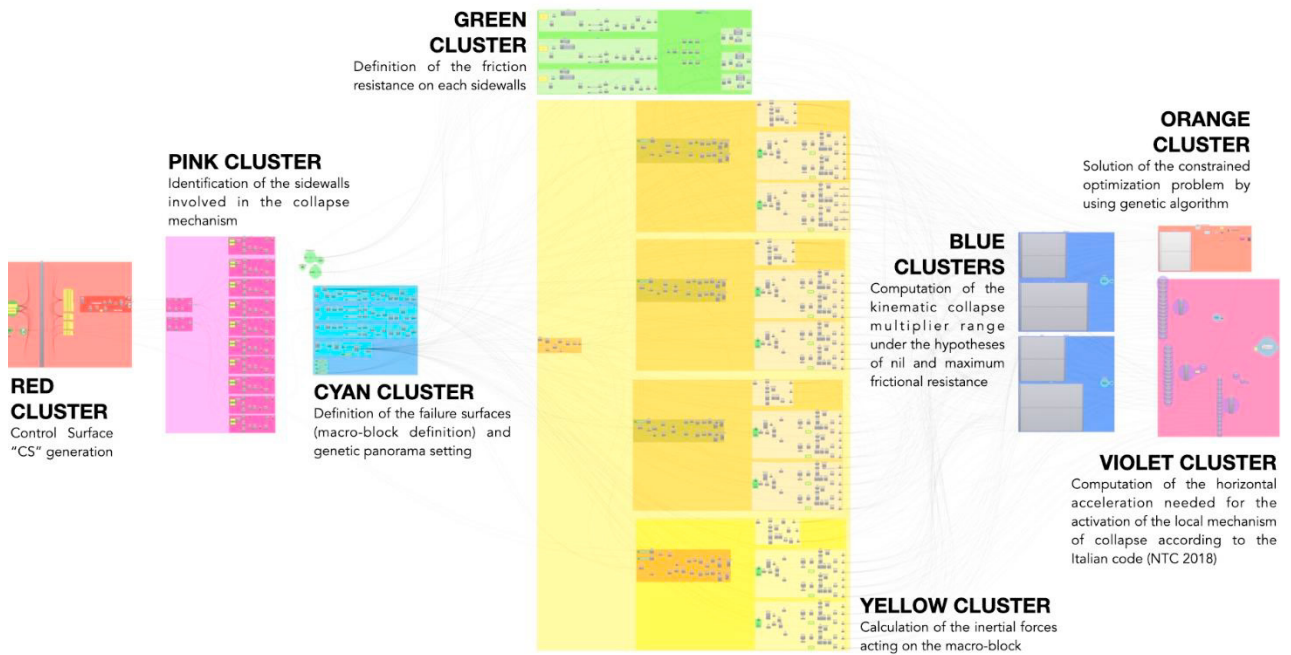
Fig. 1. Visual programming for structural assessment of out-of-plane mechanisms in historic masonry structures (Funari et al. (2020)).
