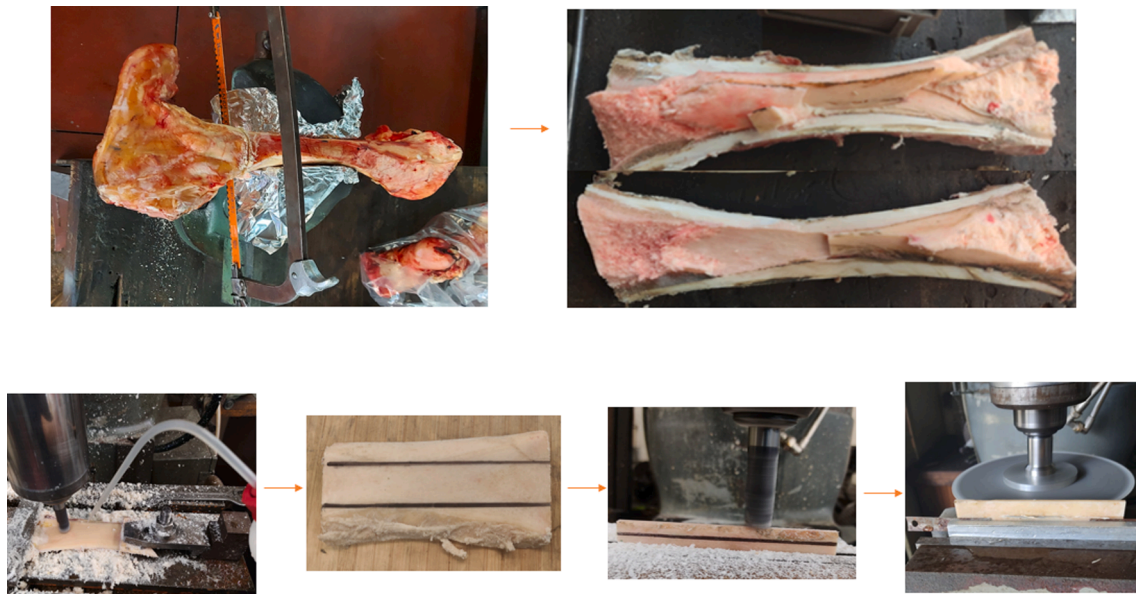
Fig. 1. Manufacturing steps of bone samples.
