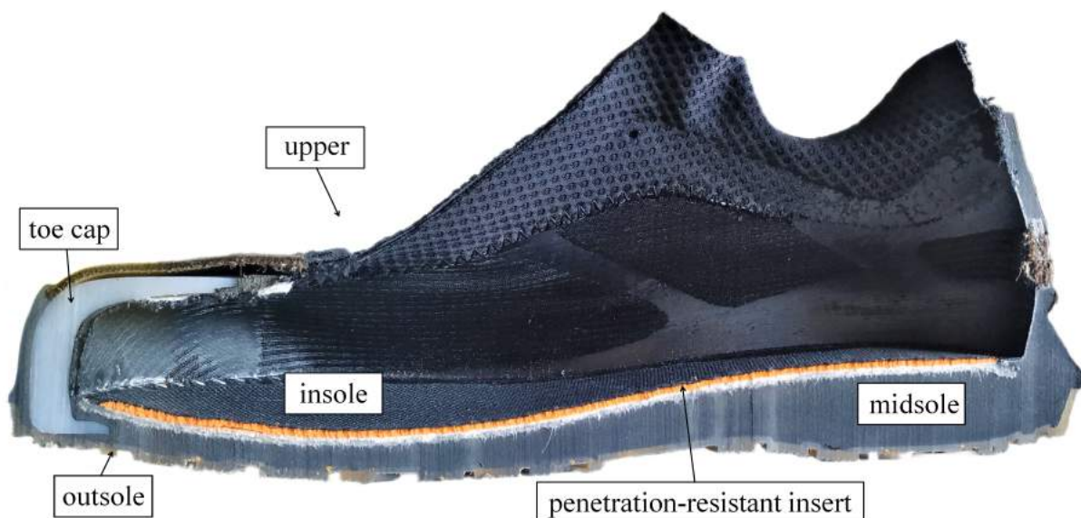
Figure 2.6: Typical construction of a safety footwear and its components.
