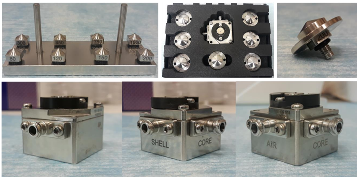
Figure 31: Internal (a) and external (b) nozzle settings, SN (c), CN (d), FVN (e), and pulsation chambers of the BUCHI Encapsulator model B-395 Pro.
