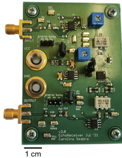
Figure A.6: Photograph of the second version of the echo receiver board.
