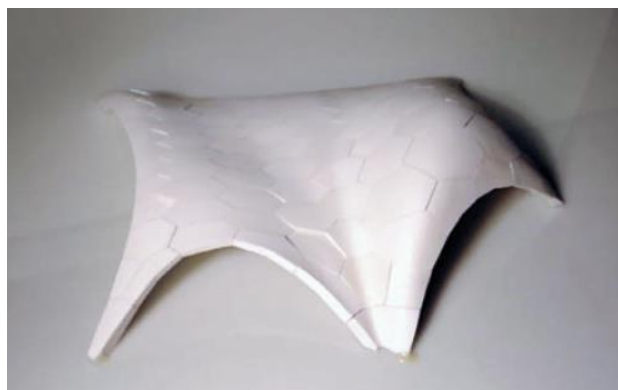
Figure 19 - 3D printed shell prototype with hexagonal tessellation (Adriaenssens et al., 2014)
