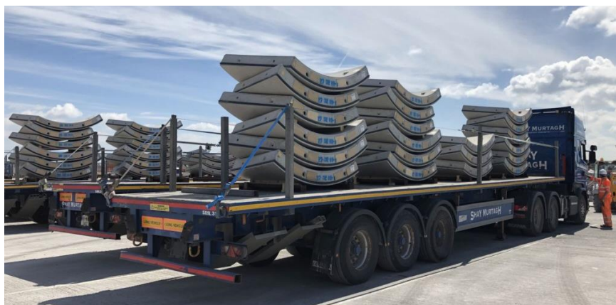
Figure 17 - Large precast concrete panels on a truck (Shay Murtagh, 2021)
