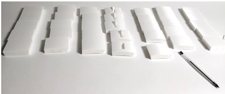
Figure 45 - 3D printed blocks before assembly
