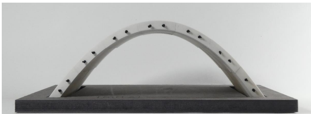
Figure 46 - 3D printed blocks after assembly - Front view
