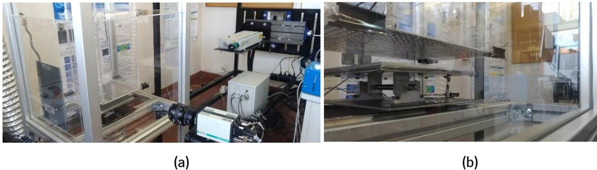
**Figure 35.** (a) PIV system; (b) measurement region.
