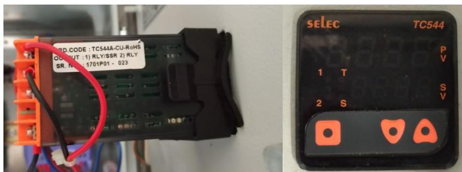
**Figure 24.** Temperature controller TC544A.
