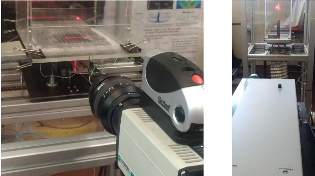
**Figure 33.** PIV system alignment using the Bushnell® laser.
