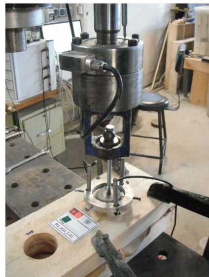
b) Pull-off test.
