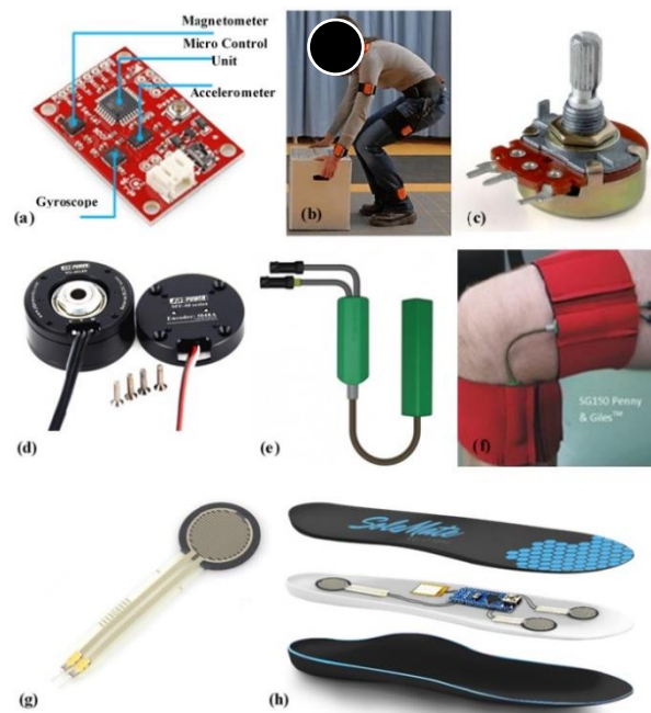
Figure 3-11 - Kinematic and kinetic sensors used in lower limb exoskeletons and AFOs: (a) IMU board integrated with its components, (b) IMU motion tracking system developed by XSens, (c) Potentiometer, (d) Encoder integrated in a DC motor, (e) Strain gauge goniometer with flexible connecting beam, by Pluxx, (f) Flexible
