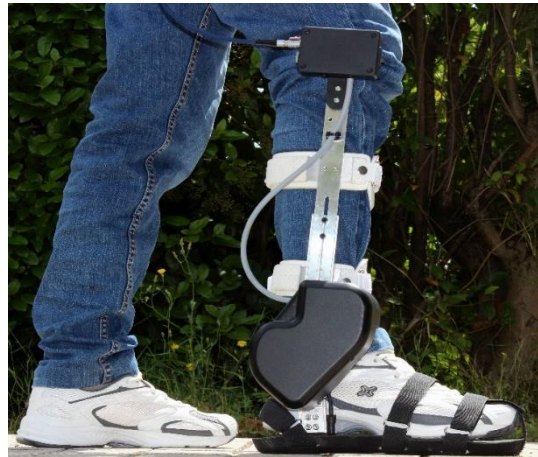
Figure 3-6 – Example of an active AFO: Ankle module of the Technaid H2 lower limb robotic exoskeleton powered by an electric motor [83].
