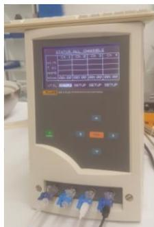
Figura 5.1 – *Fluke Biomedical IDA 4 PLUS IDA Infusion Device Analyser Series*.
