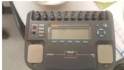
Figura 5.2 – *Fluke Biomedical Impulse 7000DP Defibrillator Transcutaneous Pacer Analyzer*.
