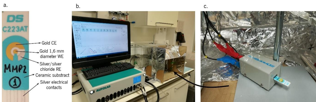
Figure 20. a. Sensor layout, b. electrochemical measurements setup and c. connector.
