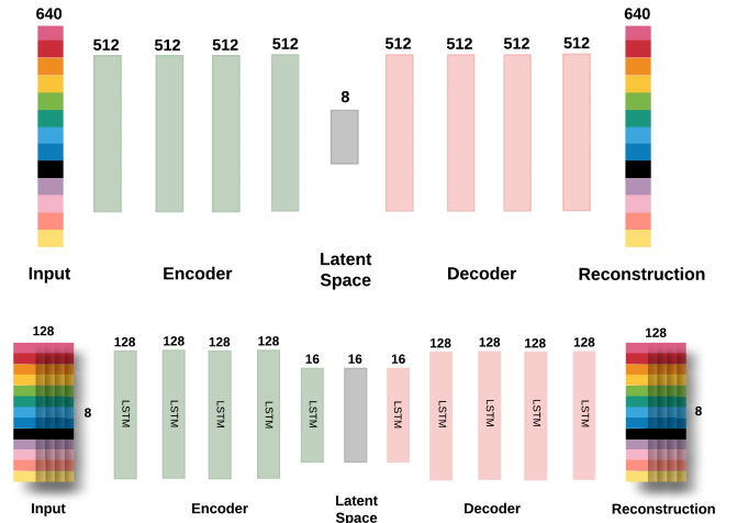
Fig. 5: Dense-AE (top) and LSTM-AE (bottom) architectures.
