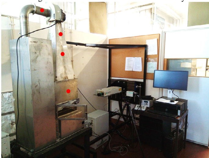
Fig. 4. Experimental apparatus and identification of the seeding zones.
