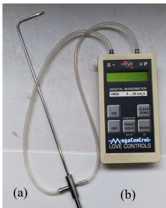
Fig. 6 - Devices for jet velocity measurement: (a) Pitot tube (b) Manometer.
