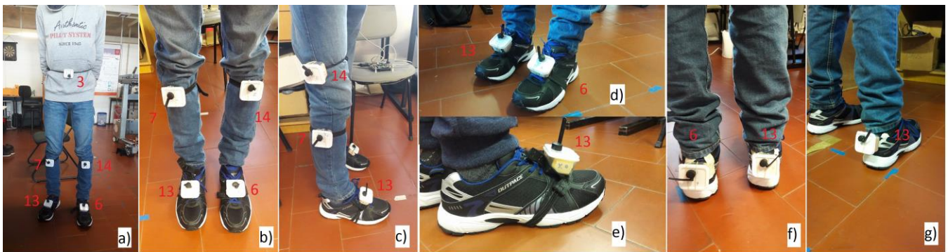
Figure 3. Spatial arrangement of the sensory modules in the body with their physical addresses: a) 5 sensory modules on trunk (3), foot (13-right, 6-left), and shank (7-right, 14-left); b) 4 sensory modules on foot (13-right, 6-left), and shank (7-right, 14-left); c) 3 sensory modules on right leg: foot (13), shank (7), and thigh (14); d) 2 sensory modules on the upper foot (13-right, 6-left); e) 1 sensory module on the upper foot (13-right); f) 2 sensory modules on the heel (13-right, 6-left); and g) 1 sensory module on the heel (13-right).
