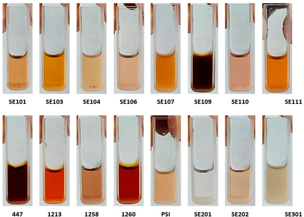
Figure 1. Colors of the synthesis reaction of silver nanoparticles with aqueous extracts of different entomopathogenic fungi.
