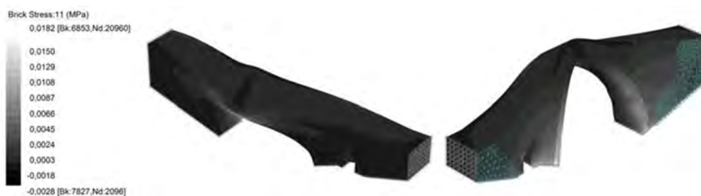
Fig. 11. Principal tensile stress contour for the elastic response spectrum analysis.
