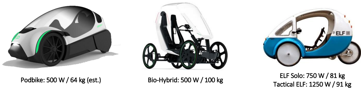
Figure 4: Examples of human-powered electric vehicles of recent design (left to right): Sørensen’s Podbike, Schaeffler’s Bio-Hybrid and Organic Transit ELF, shown with their assistance power and mass parameters.
