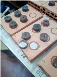
Mortar with the metal disc on the brick substrate
