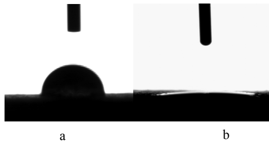
Figure 4. Static contact angles of water drop on a) Sample of original polyester; b) Hydrolyzed PET with PEG (250 g/L, M_w 2000) and resin (60 g/L) by pad-dry-cure process.
