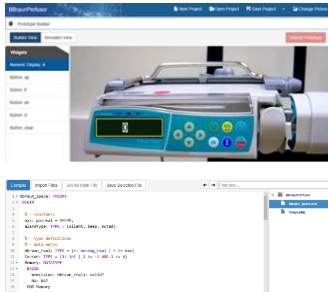
Figure 67. Screenshots of the main tools provided by the PVSio-web environment. Top image – Prototype builder; Bottom image - model Editor and a model snippet generated from emuchart editors.
