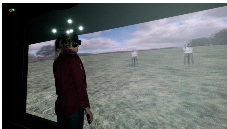
Figure 47. FMDT in the IVE conditions. Participant performing the FMDT in the IVEPH condition. The structure with retroreflective markers on the participant's head is used in order to track participant's head position and rotation.
