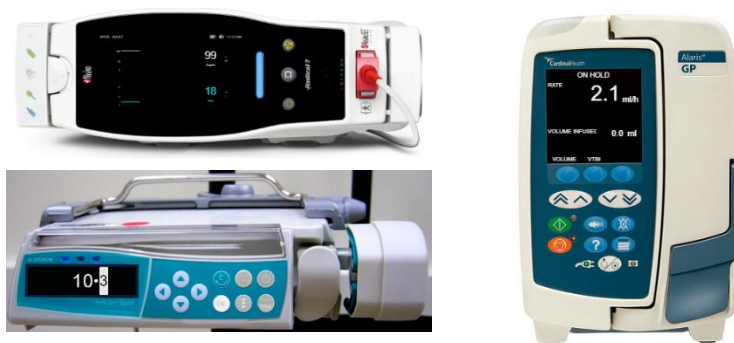
Figure 74. Medical devices currently modeled and available in our SBME. The top-left one is the Massimo Radical 7® Pulse Co-Oximeter® a monitoring device that keeps track of patients oxygen saturation, pulse rate, and perforation index; the bottom-left one is the BBraun® Infusionmat IV Pump, a programmable syringe based infusion pump; the right one is the Alaris® GP Volumetric Pump an infusion pump suited for drugs therapy, blood transfusions, and parenteral feeding
