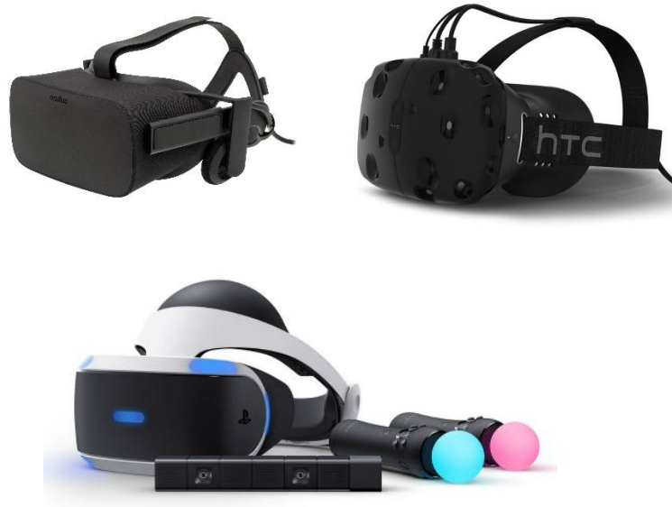
Figure 25. PC-based premium HMDs currently commercially available. Top-Left is the Oculus Rift Consumer Version 1; top-right is the HTC Vive; down is the PlayStation VR from Sony (images distributed under a CC-BY 2.0 license).
