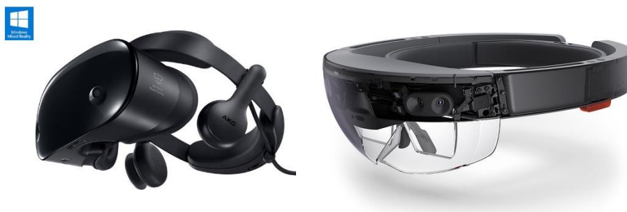
Figure 25. The Samsung Odyssey and the Microsoft HoloLens, two of the state-of-the-art equipment for mixed reality and augmented reality.
