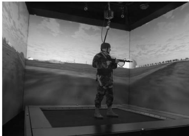
Figure 26. A CAVE visualization system with an omnidirectional treadmill from the U.S. Army Research Lab. From [88]
