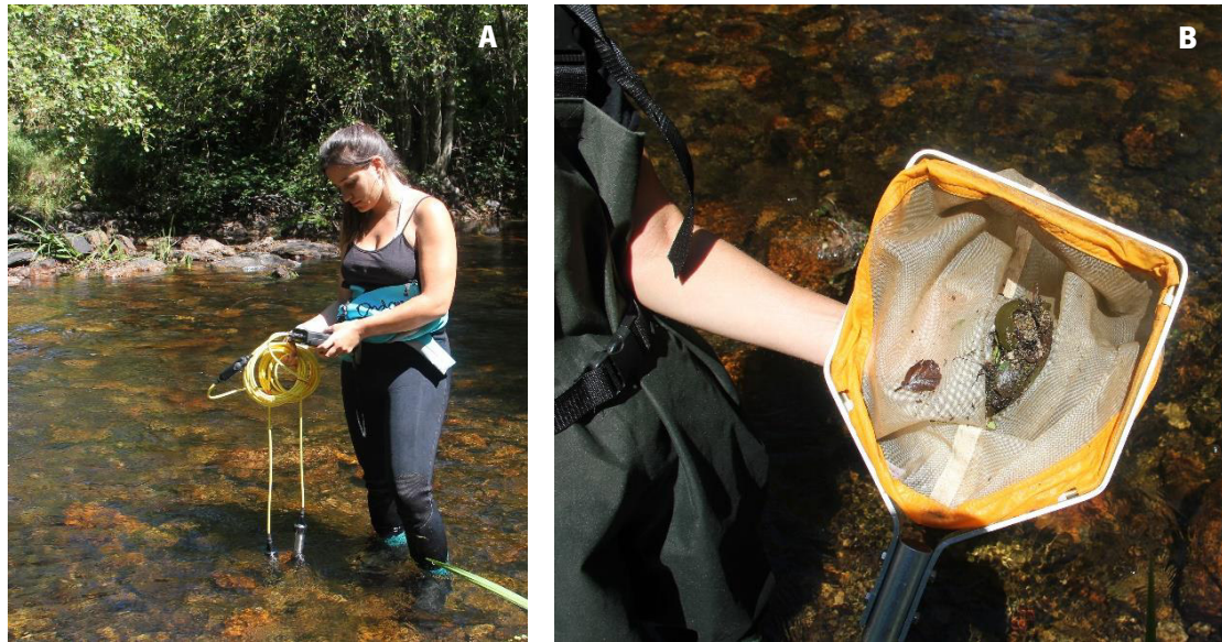
Figure 6 – Measurement of abiotic variables with a multi-parameter probe (A) and hand net used to collect the macroinvertebrates (B). Courtesy of Ronaldo Sousa.
